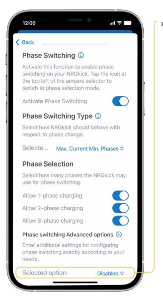
Disabled: The Phases switch over as quickly as possible.
