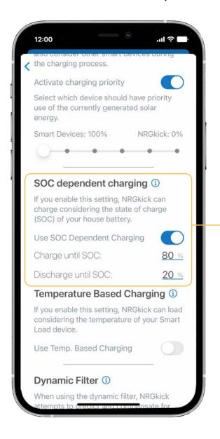
» SOC (State of Charge) dependant charging: With this setting, you can define a state of charge limit for the house battery if required. After exceeding this limit, the charging power of the house battery is withdrawn and diverted to the NRGkick.
