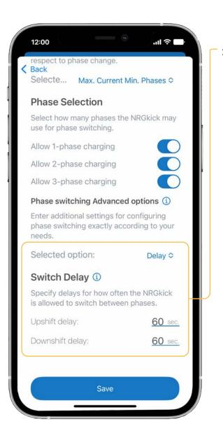
Delay: An up-switching and downswitching delay time can be defined here. For the phase switch to take place, the specified power must exceed the power limit that applies to the number of phases for the specified time period.
