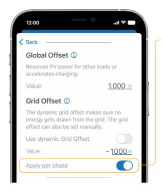
Additionally you can define if the grid offset is applied per active load phase. This is especially useful for phase switching, because the number of phases, changes at runtime.
