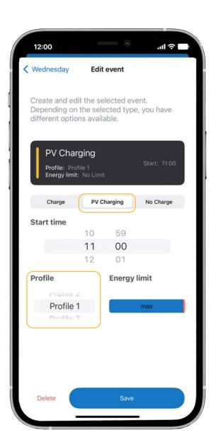
**4.2.** Using the "Add event" button, PV charging can now also be set and various PV profiles can also be selected.
