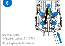
Recommended conductor cross-section for screw terminal connections: 2.5 - 10 mm<sup>2</sup>
