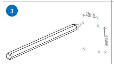
Mark the drill holes as indicated in the picture. Alternatively, you can use the bottom part as a "template". Then drill the holes according to the markings.
