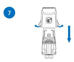
Place the top part on the bottom part. Bend the two lowest points of the upper part slightly outwards. Make sure that the guide rail of the top part is correctly inserted into the bottom part and then push the top part down until the locking hooks engage.
