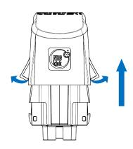
The top and the bottom part of the wall socket are taken apart as follows: Pull the lower ends of the top part slightly outwards as described in the picture so that it can be removed from the bottom part.
