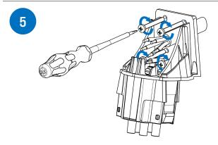
Attach the bottom part to the wall at the four points provided for this purpose (make sure it is properly attached according to the wall structure).
