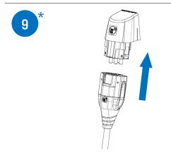
Connect the NRGkick charging unit to the Wall Socket.
