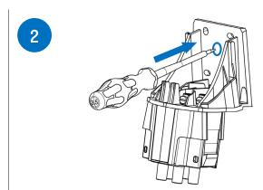
There is a pre-punched opening on the backside of the bottom part of the Wall Socket. This opening can be pressed or drilled out using a suitable tool. The opening can be sealed with the help of the stepped nipple.\*\*
