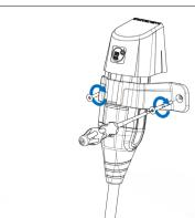
Return the locking latch to the position described previously and mount it to the wall at the two points provided for this purpose (make sure it is fastened properly according to the wall structure).
