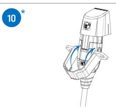
Align the locking latch so that the locking pins are placed at the bottom. Then insert the two locking pins into the holes of the connector unit.
