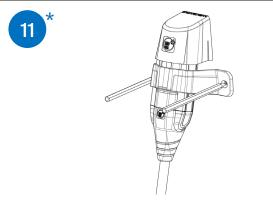
Make a mark at the two holes of the locking latch. Then remove the locking latch and drill the holes at the markings.
