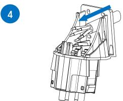
Insert the supply line through the opening.
