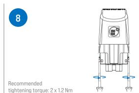
Connect the top part and bottom part of the Wall Socket using the screws supplied.
